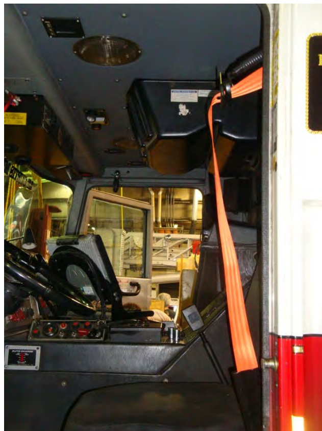
The increased length of the stalk of the ReadyReach seat belt helps to accommodate the increased size of a firefighter in bunker gear.
