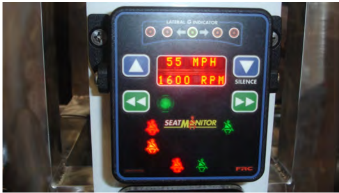
A digital display on a vehicle data recorder (VDR) gives the operator and the officer a variety of safety information about the apparatus and the onboard personnel.
