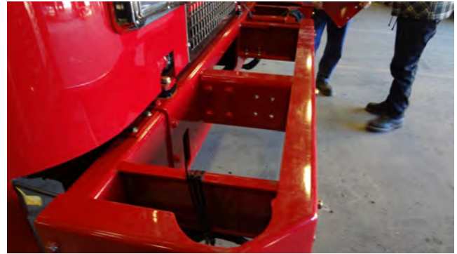
Steel reinforced front bumpers have become a popular option to protect the crew from cab intrusion.
